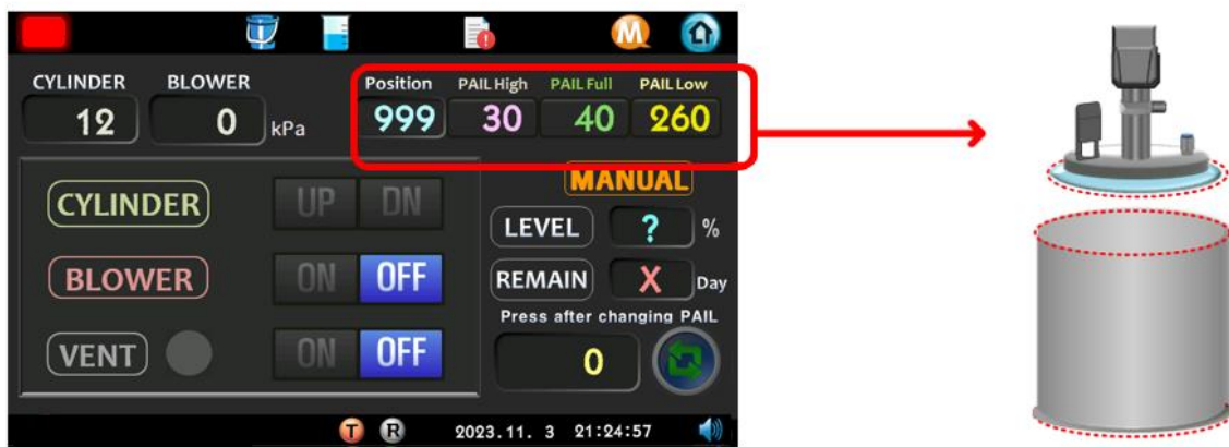
Figure 11. Cylinder position value at initial container setting
