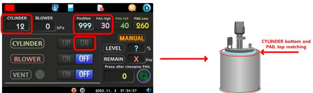
Figure 13. Container top set-up
